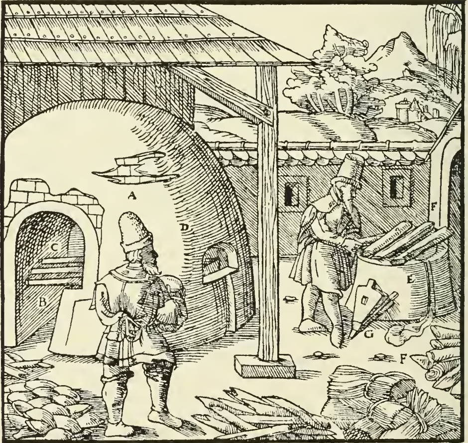
A—FURNACE SIMILAR TO AN OVEN. B—PASSAGE C—IRON BARS. D—HOLE THROUGH WHICH THE LITHARGE IS DRAWN OUT. E—CRUCIBLE WHICH LACKS A DOME. F—THICK STICKS. G—BELLOWS
